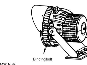
A:Fix the M20bolt at the mounting surface plate
